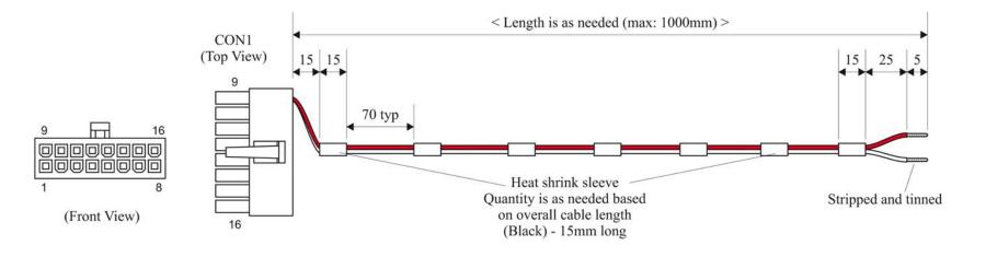
Terminal<br/>CON1Housing<br/>Leotronics 6740-1160<br/>(2x8way 4.2mm pitch with latch, 6A de-rated)Crimp<br/>6744-2000<br/>(tin plated, female)
