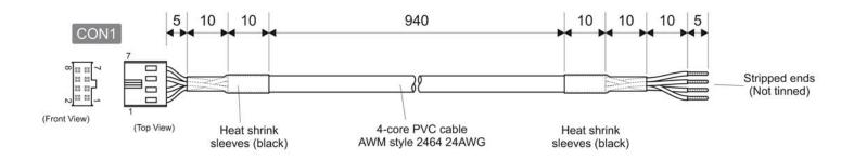
**Terminal** Housing Molex 90142-0008 (2x4way 2.54mm pitch with key)
