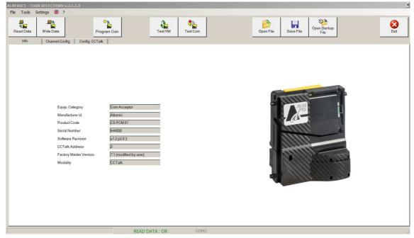
Click on the tag 'Channel Config.' to read the programmed channels.
