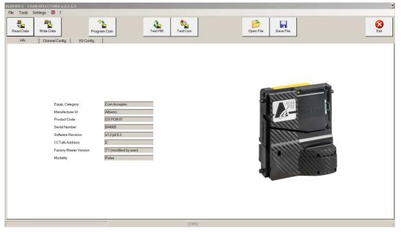
The acceptor identifying data will appear beside the image of the acceptor. If the coin acceptor has been set to Pulse operation (see Chapter 2. USING THE DIP SWITCH ROWS), the third tag will show 'I/O Config.', as it appears in the example picture above. If instead the coin acceptor has been set to ccTalk operation, the third tag will show 'Config.' CCTalk'as it appears in the example picture below (referring to an AL66 FG acceptor).
