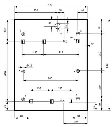
Prepare the tunnel for the power cable in the wall (corresponding to "Y" Hole in the slab).
