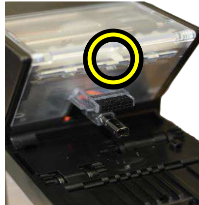
Normal tape position – diverter in CLOSED
