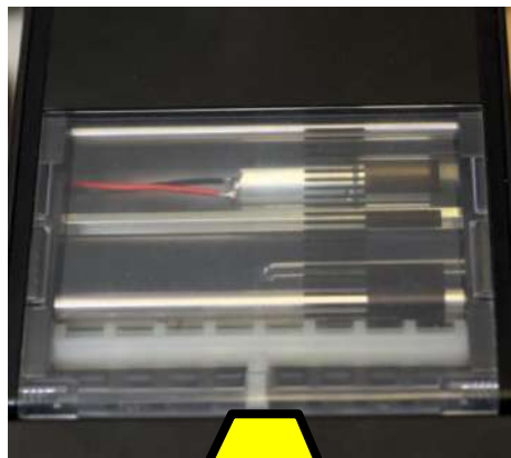
Normal tape position – diverter in CLOSED
