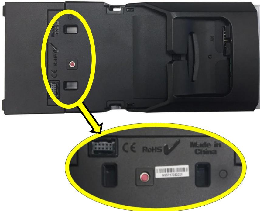
Once the Multi Notefloat is attached the configuration button on the NV9 Spectral is not accessible. Use the configuration button on the front of the Multi Notefloat.
