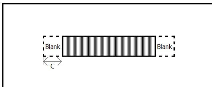
A blank space (C) is required on either side of the barcode as pictures or text may be seen as part of the barcode value.
