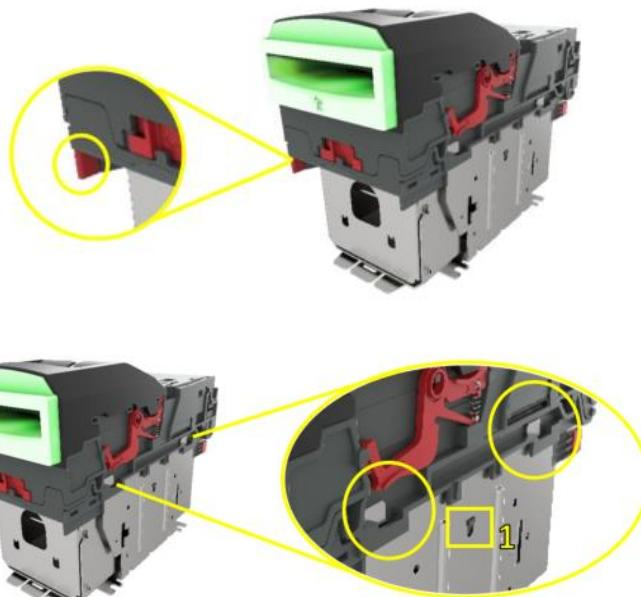
Push the tab (1) seen in the image whilst sliding the outer housing back, so that the locating tabs are free to move away from the validator.
